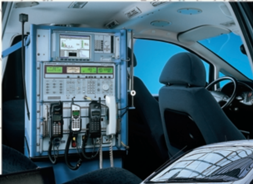
FIG 1 TS995 x offers an extensive line of products for mobile-radio networks covering practically all fields of application: network planning, installation, optimization and monitoring. The example below shows portable system TS9951 (case) and high-performance test system TS9955 (vehicle).
